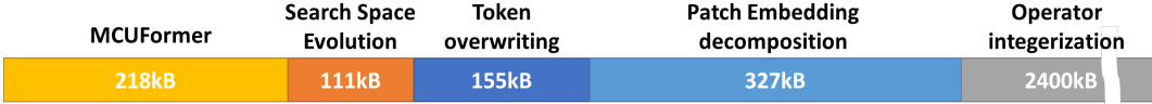
Figure 3: The peak memory reduction is achieved through the operator library with memory scheduling techniques, including patch embedding decomposition, Operator integration, and token overwriting. The peak memory of the final model adheres to the SRAM constraint, which is 256kB.
